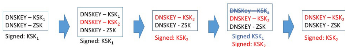
Figure 3 – Root Zone KSK Roll – after RFC5011
